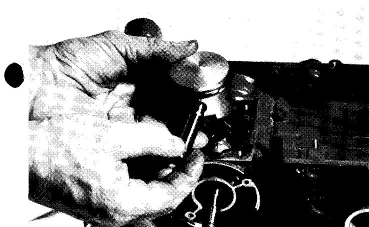
**Fitting the piston and cylinder to the engine block**
