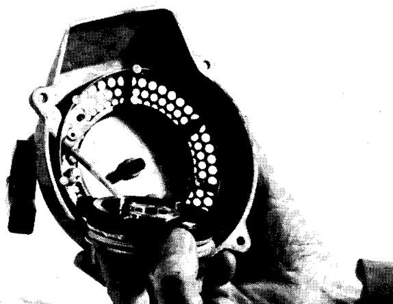
**Fig. 6** First place the large washer in the fan housing. Fit the spring and the magazine on the cord drum. Lay as much of the cord as possible in the drum slot. The drum, spring and magazine can now be placed in the fan housing.
