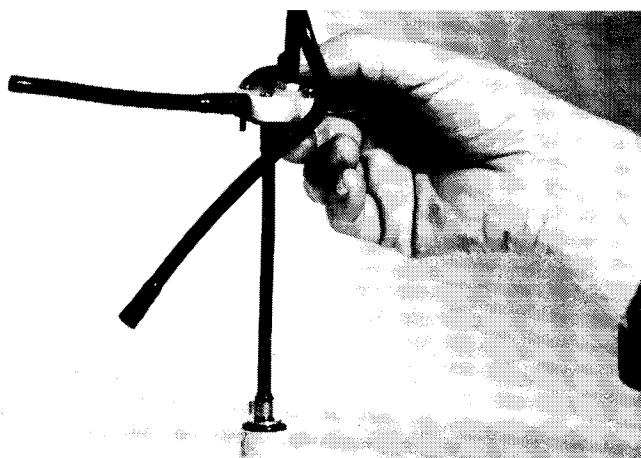
**Fig. 42** The hose connection. Check valve and hoses. If the filter in the plummet hose requires replacement, it is unnecessary to unscrew the relief valve. The plummet hose can be reached through the fuel filler hole. A comparison can be made by blowing through a new and an old plummet hose assembly to find out whether it is allowing enough fuel to pass through.
