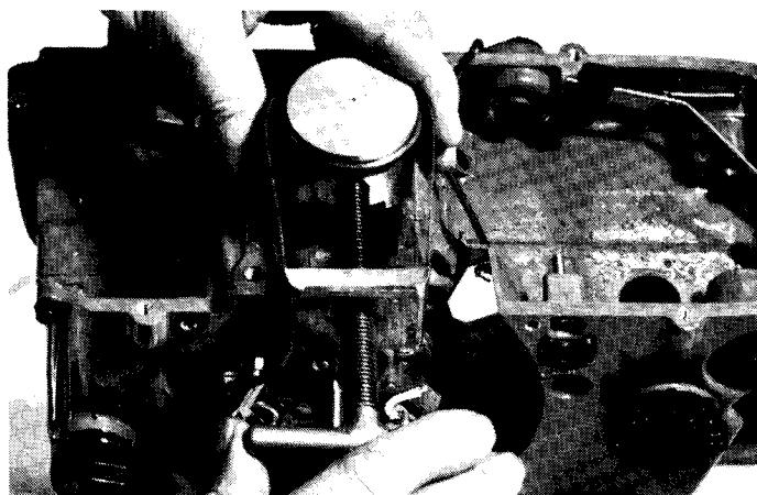
**Fig. 23** Remove the cylinder head, fan housing, silencer (muffler), the fuel hose attachment at the carburetor, the split pin at the choke control, and the intermediary section.
